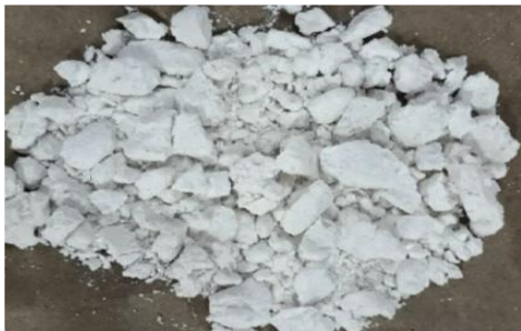
Struvite product B with Molar ratio of (\text{PO}_4)_3 : \text{Mg}^{2+} : \text{NH}_4^+ = 1: 2: 4
